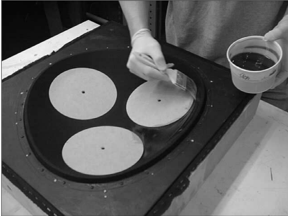
Applying fiberglass resin to the cloth.
