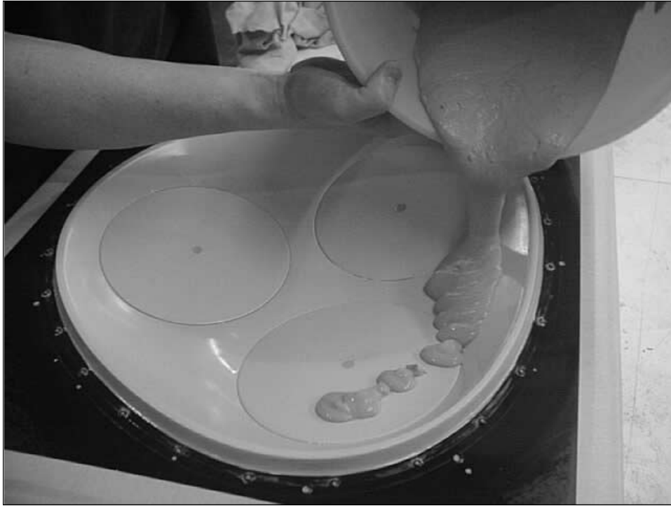
Pouring the plaster onto the plug.
