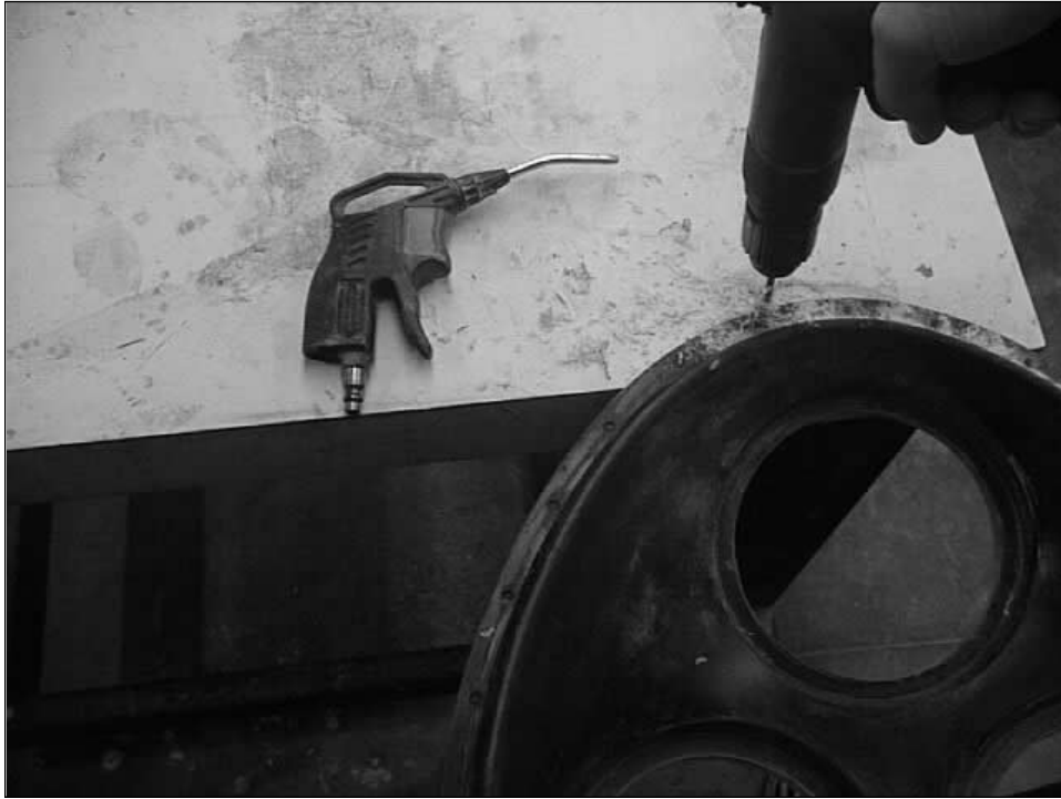
Drilling out the mounting holes.
