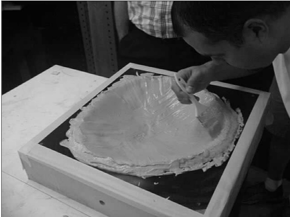
We brushed the plaster from the center of the plug/model outward. This will prevent the plaster from sliding, causing a flawed mold.
