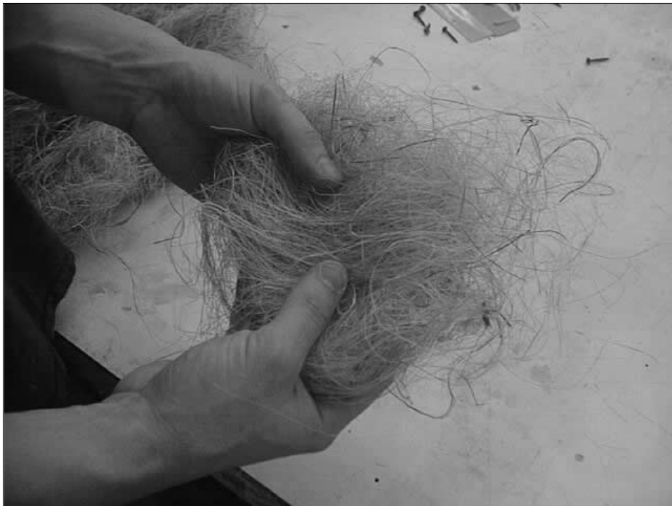
We made enough hemp patties to cover the entire surface of the plug/model. The hemp patties will reinforce the plaster mold when it dries.
