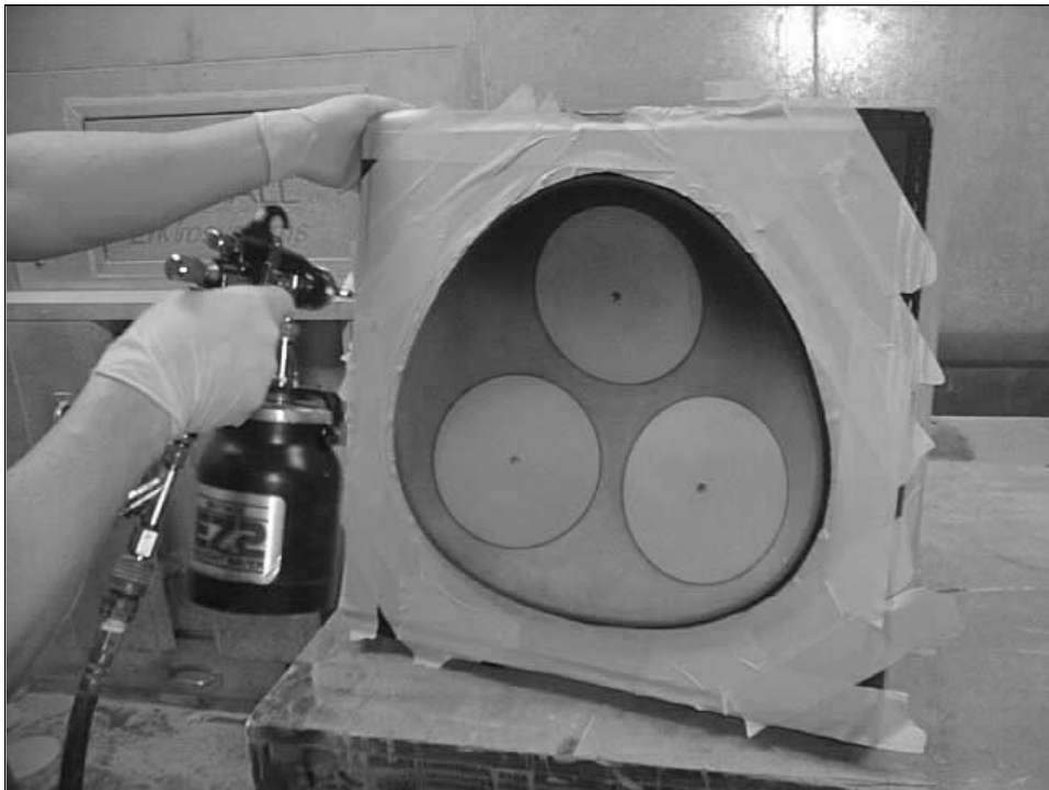
Applying the primer fill with a spray gun.
