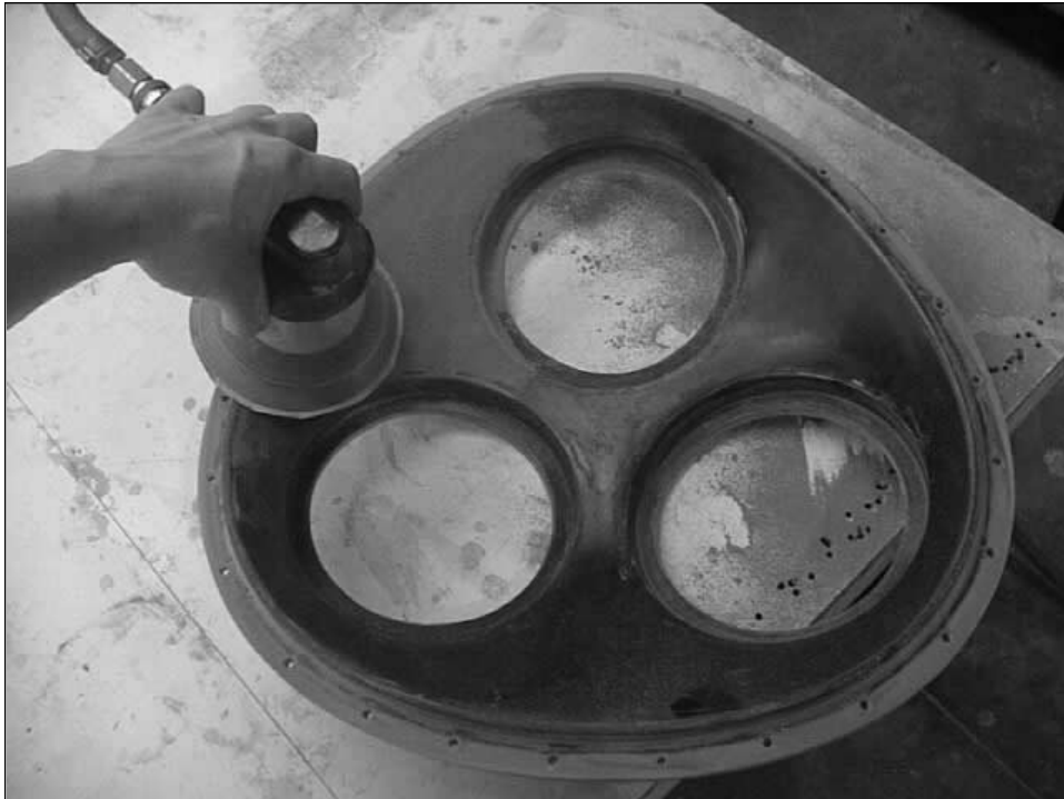
Sanding the fiberglass plate with 150 grit sand paper.
