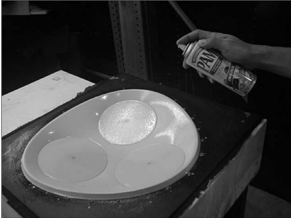
Spraying a coat of Pam on the plug/model as a release agent.
