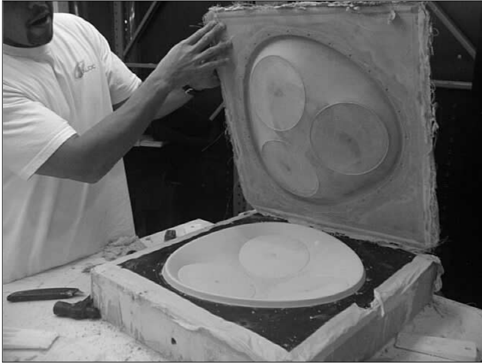
Removing the plaster mold away from the plug.
