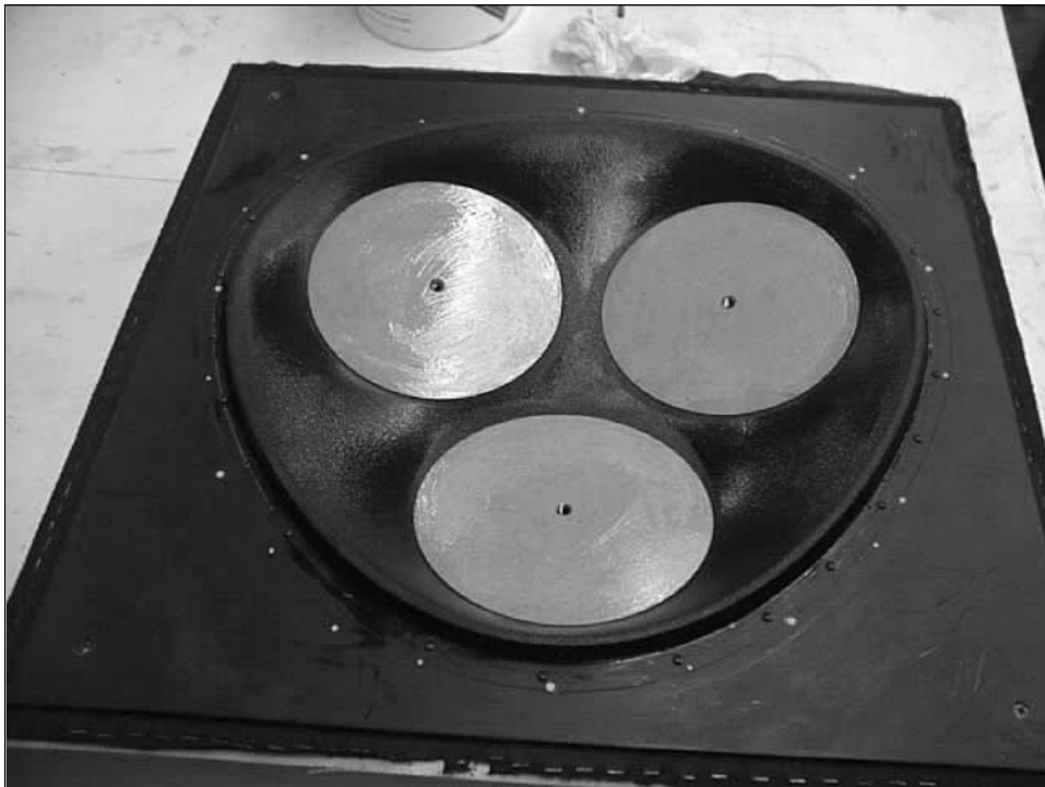
After the resin hardens, the plug/model is ready for the next step.
