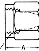
Versil·Flare™ Flareless Tube Nut Part No. FC2875-(Dash size) Use with FF9605-(Dash size) Ferrule Only
